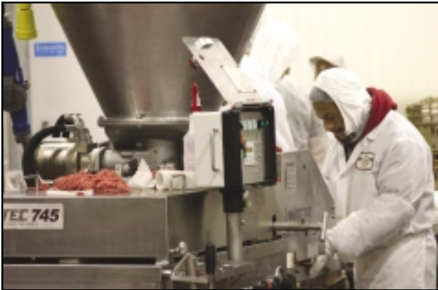
A new patty former folds rather than molds meat into shape. (Photo courtesy Prizm Group.)
